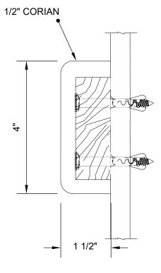
Use 1/8" continuous bead of 100% silicone adhesive to attached bumper to substrate. Support to avoid slippage during setup.
